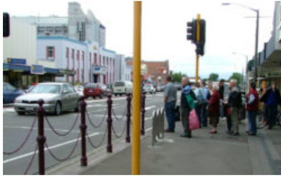
Figur 6: Signalregulert gangfelt, Palmerstone North, New Zealand. Merk stengsler for å unngå kryssing utenom gangfeltet (NZ Transport Agency 2009, Foto: S. Turner).
